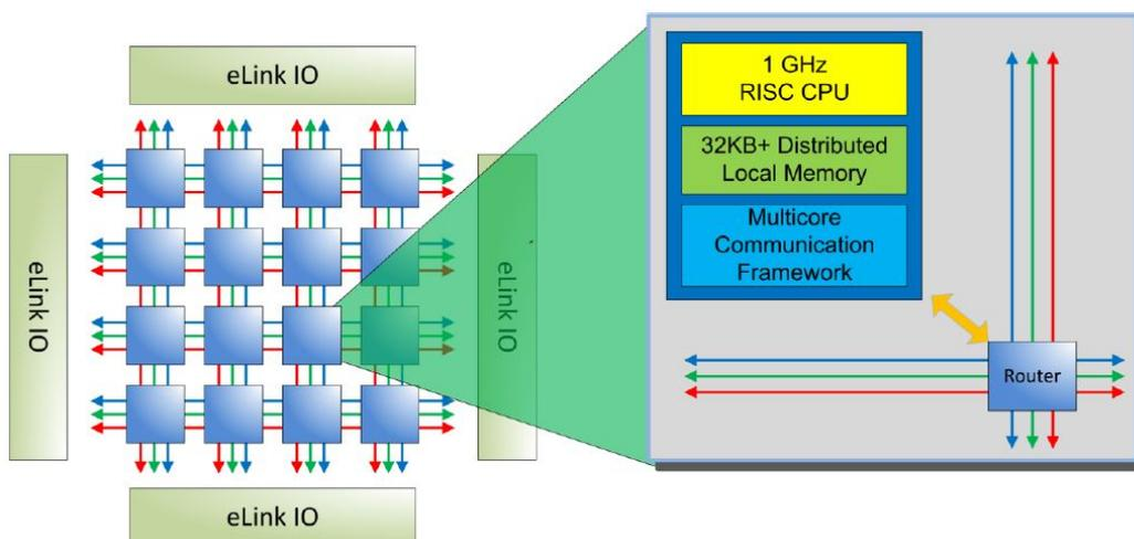
Figure 3.2: Layout of the Epiphany chip from [5]
