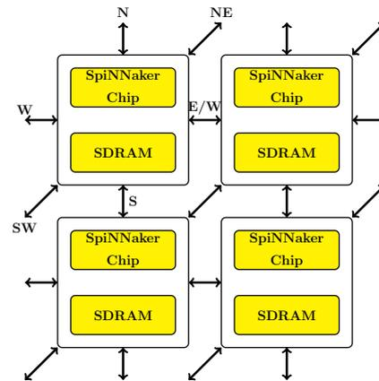
Figure 2.2: Hexagon layout of the chips from [6] and [18]
