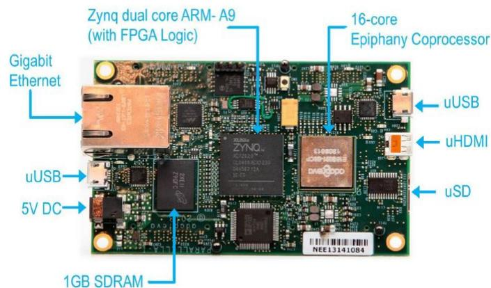
Figure 3.1: The Parallella Board taken from the Reference Manual [3]
