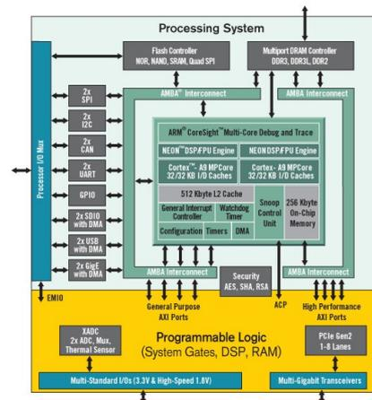
Figure 3.4: Layout of the used Zynq
