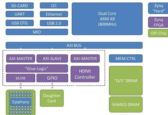
Figure 3.3: The Parallella Board Architecture from the Reference Manual [3]
