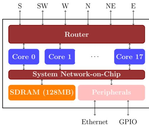
Figure 2.1: Architecture of a SpiNNaker node from [10]
