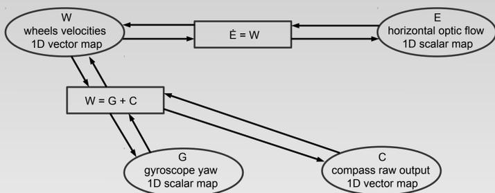
Fig. 4 Orientation detection network architecture for a mobile robot
